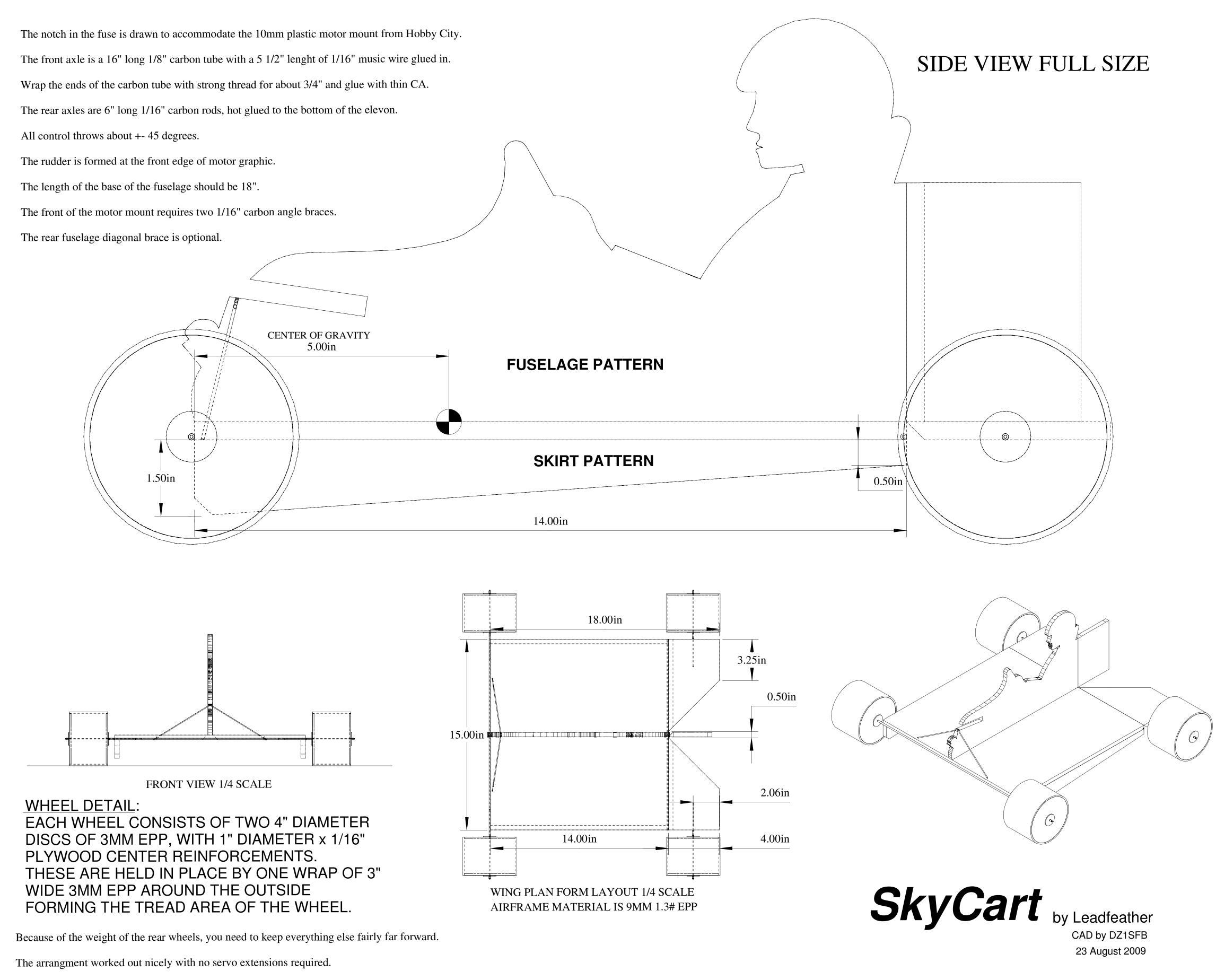
9 gram servos for the elevons, 5 gram for the rudder. This arrangement got the battery right about at the cg.
